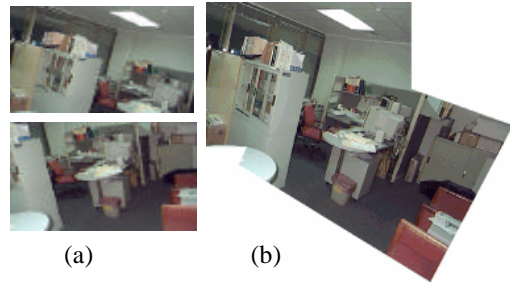
Fig. 6: Stitching result when the camera has rotation changes.
