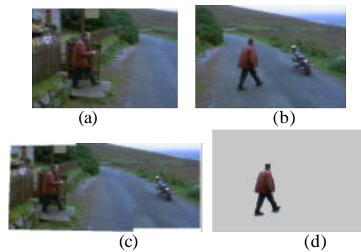
Fig. 7: Mosaic construction and object detection. (c) is the mosaic result of (a) and (b). (d) is the object detection result by image differencing.
