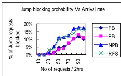
Fig. 16. The blocking probability of forward jump function vs. user arrival rate.
