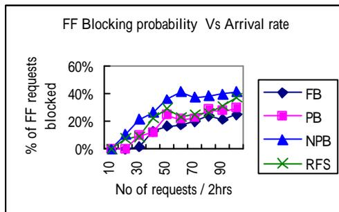
Fig. 15. The blocking probability of fast forward function vs. user arrival rate.
