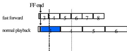
Fig. 3. The ending time of executing fast forward function belongs to the first one section of some time slot.
