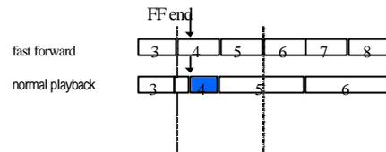
Fig. 4. The ending time of executing fast forward function belongs to the second one section of some time slot.
