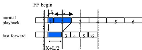
Fig. 2. The beginning time of executing fast forward function belongs to the second one section of some time slot.
