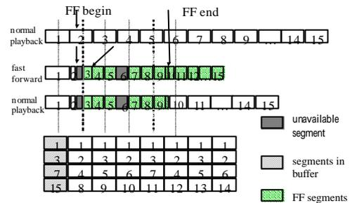
Fig. 5. The situation that the beginning time of executing fast forward function belongs to the first one section of time slot two and the ending time of executing fast forward function belongs to the first one section of time slot six.
