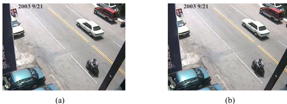
Fig. 7. (a) Original authentication frame, by H.263, QP=7, bit-streams=12169 Bytes, (b) Watermarked frame, PSNR=42.5db and bit-streams=12378 Bytes
