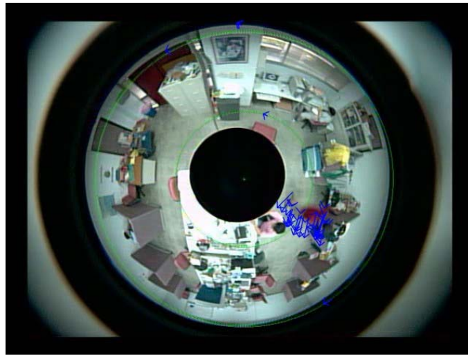
Fig. 5. Tracking result using optical flow. The vectors represent the image gradient change above a threshold.
