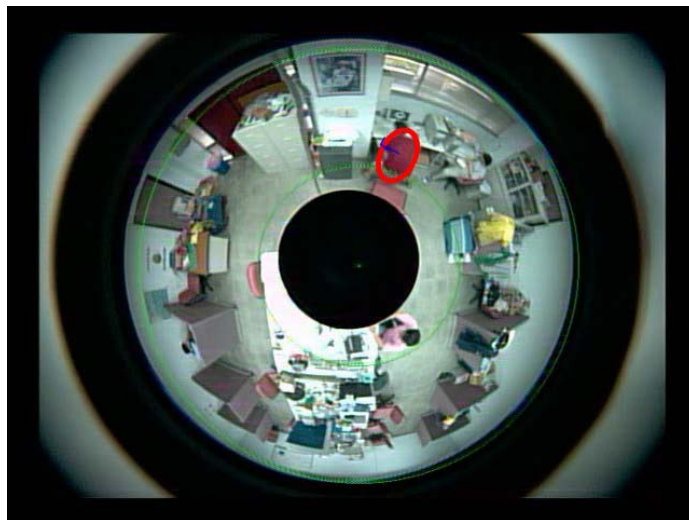
Fig. 6. Tracking result from the combination of both methods. CamShift is represented by a red ellipse and optical flow is represented by a blue vector.
