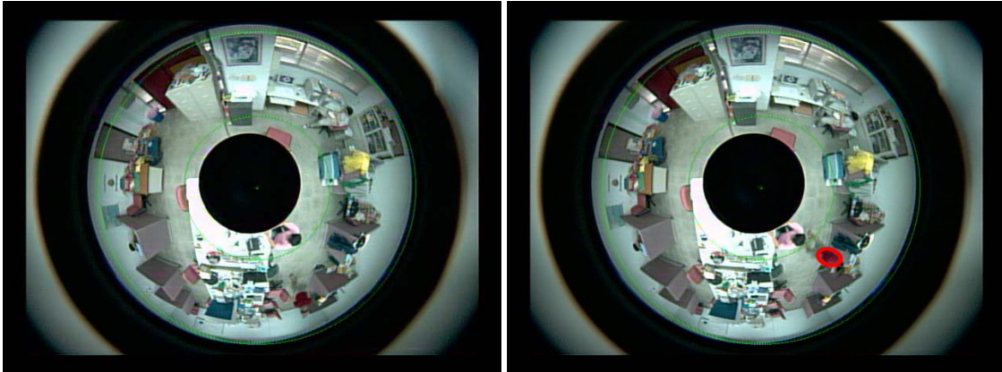
Fig. 4. The left image shown the original image. The right image is the tracking result using CamShift algorithm. The tracked target is shown by a red ellipse. The axes can be used to represent the direction of the motion.
