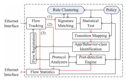
Fig. 2. Design of online application and behavior identification
