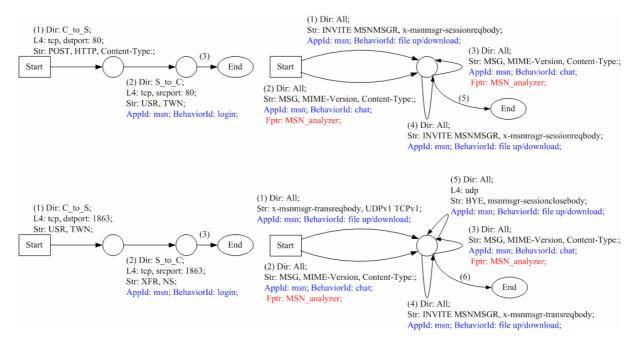
Fig. 6. Two sets of MSN FAs for the official communication and for HTTP tunneling
