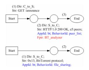
Fig. 5. The BitTorrent FAs for capturing the peer list
