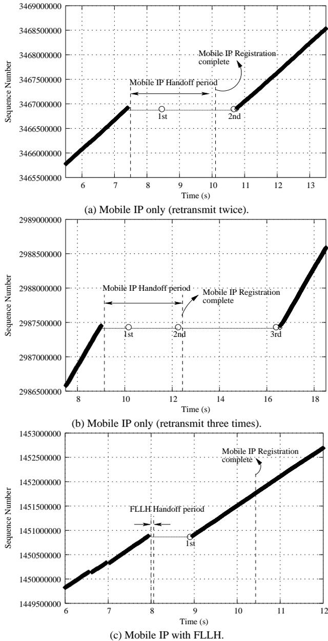
Fig. 7. TCP Packet Transmission Experiment.
