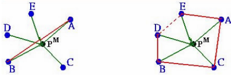
Figure 13. (a) The inserted \overline{AB} is not legal and (b) P^M 's 1-ring cyclic structure is established by inserting several legal edges.
