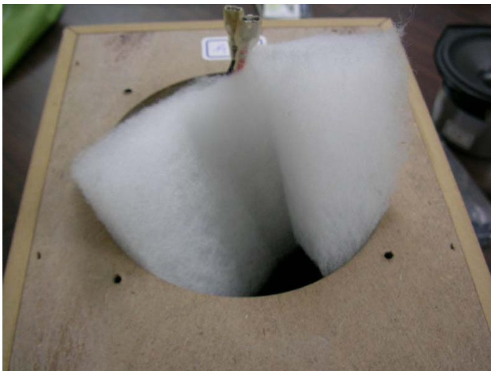
Fig.9 箱體安置吸音棉
