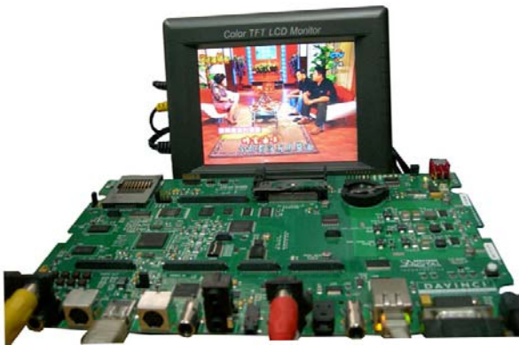
Figure 7. DM6446 broadcasting digital TV programs
