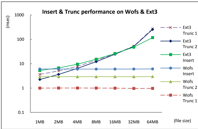
Figure 4-4. The time needed for doing 1 insertion and 1 truncation on Wofs with different file sizes ignoring the time needed for network communication, and the time needed for doing 1 insertion and 1 truncation on ext3 with different file sizes.
