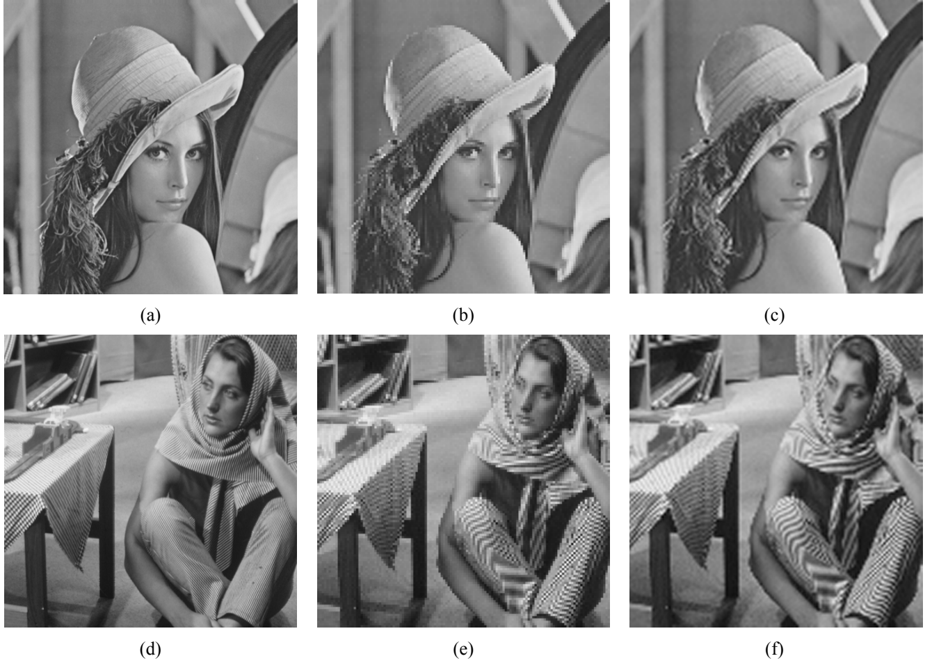
Fig. 5 The comparison of enlarged results. (a) and (d) are the original images, the rest of images are obtained from down sampled images then enlarged such that (b) and (e) are done by duplication; (c) and (f) are done by the bicubic interpolation.
