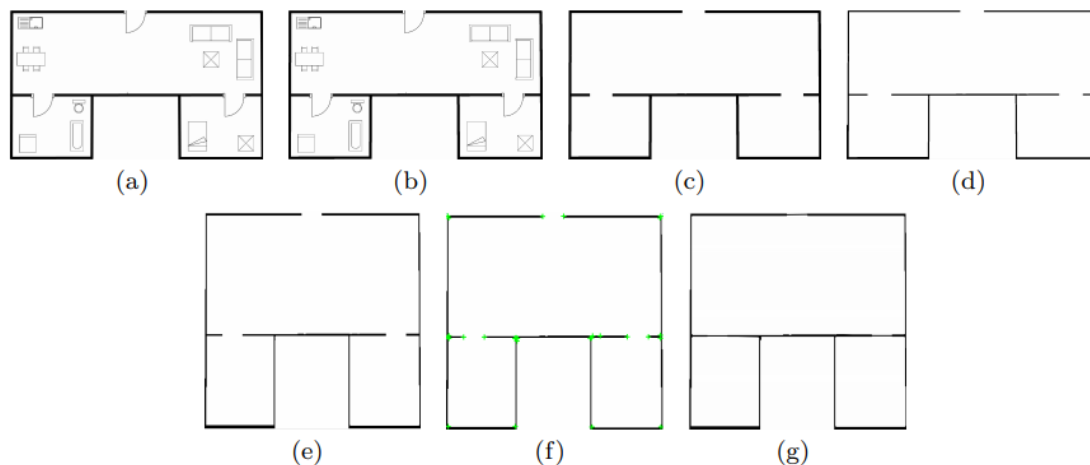
Fig. 3: Output generated after performing each image transformation process: (a) original image; (b) pixel binarization; (c) wall extraction; (d) image dilation; (e) image resize to 400 \times 400 ; (f) edge detection using FAST algorithm, and; (g) door gaps linking
