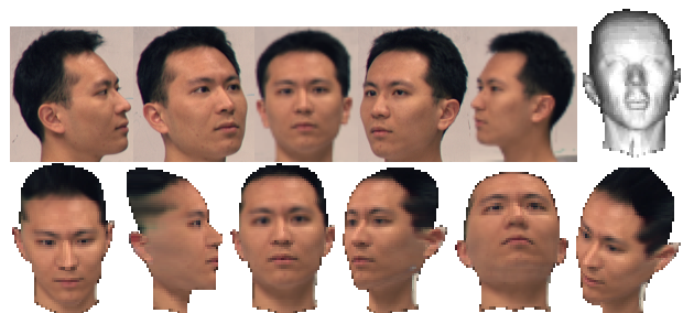
Figure 15. The upper row shows the five images of Mr. Chen and the reconstructed face model of him. Some texture-mapped results of the reconstructed model observed from different viewing directions are shown in the lower row.
