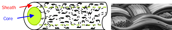
(a) Schematic of hollow filament (b) Hollow fabric Fig. 1. Schematic of hollow filament and fabric
